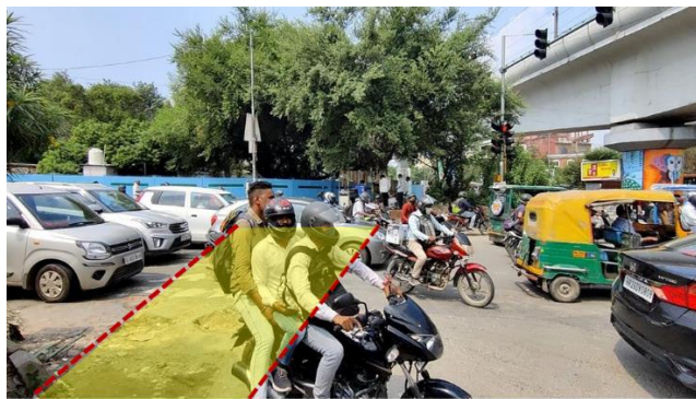
Absence of STOP line due to which vehicular traffic is coming over the junction
