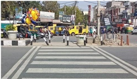
Inappropriate gap between bollards
