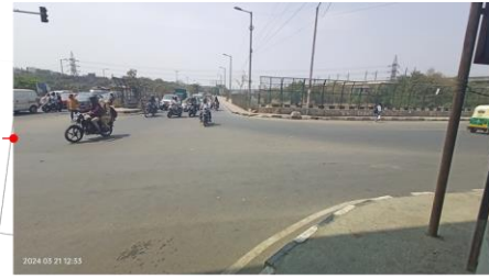
Absence of zebra crossing, kerb ramp and bollards at junction
